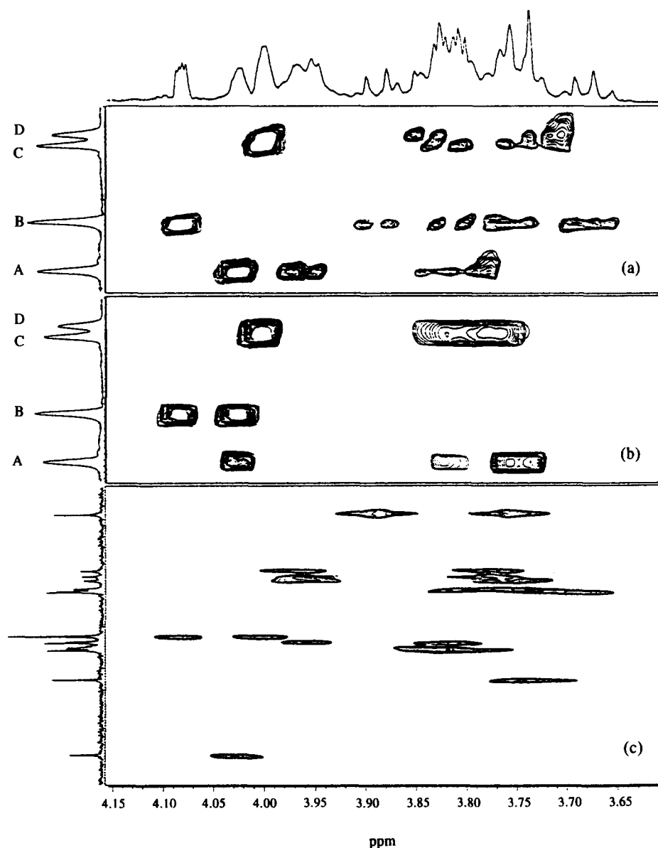
Fig. 2. 2D-NMR spectra (40°C, 500 MHz) for selected regions of the F1S-B mannan from M. gypseum : (a) TOCSY (HOHAHA); (b) NOESY; (c) HMQC subspectra. The anomeric protons have been labelled A–D.
